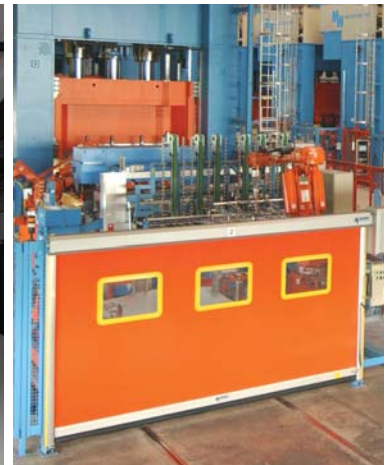
Doors for process applications - protect people, product and processes. Operating in close proximity to machinery.
